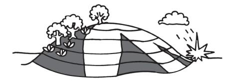
Figure 1.19 Contour lines drawn on a hill to show the areas that are level
