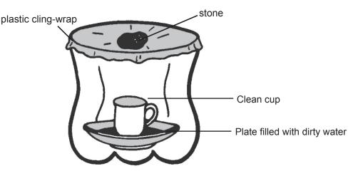
A. An evaporation/condensation chamber to simulate the water cycle.
