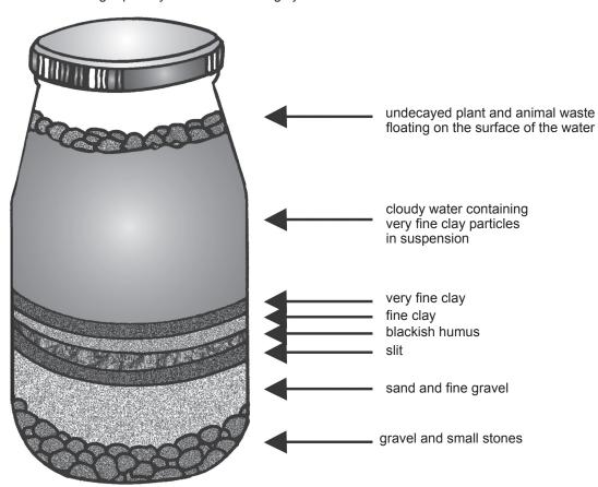
bottle in which a soil sample mixed with a large quantity of water is thoroughly shaken
