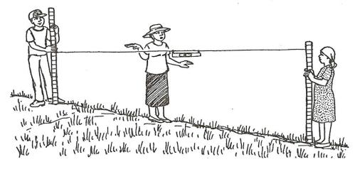
Figure 3.7 How to measure slope with a line level
