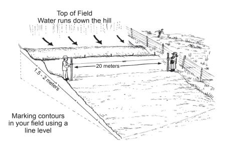
Figure 3.6 How to mark contours in a field
