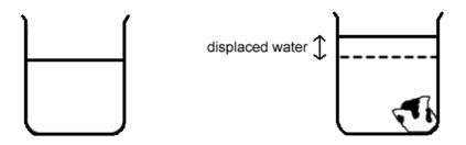
The amount of water displaced will equal the volume of the submerged stone.
