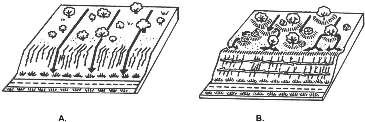
**Figure 3.13 Rill Erosion**
