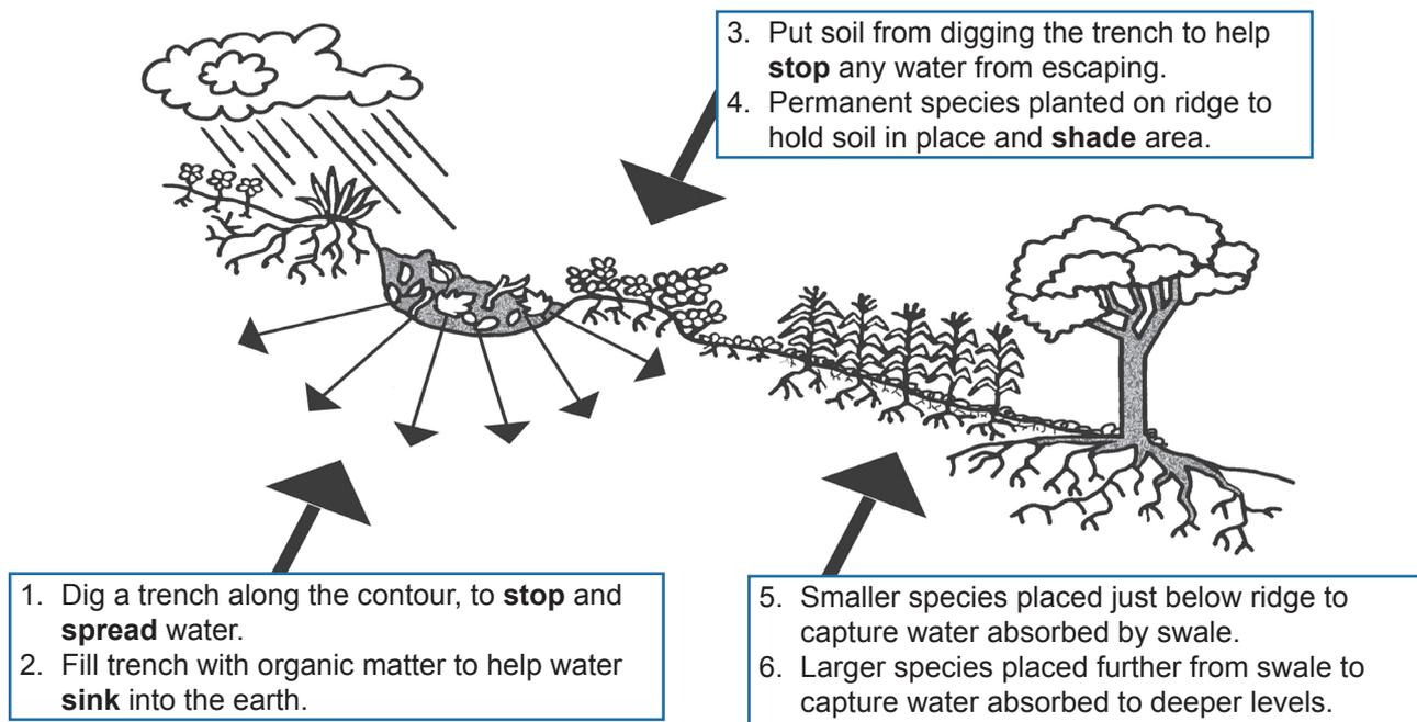
**Figure 3.3 Water-wise with swales** (Low Input, p 85)
