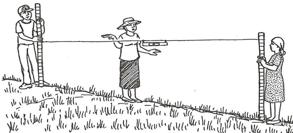
**Figure 3.7 How to measure slope with a line level**
