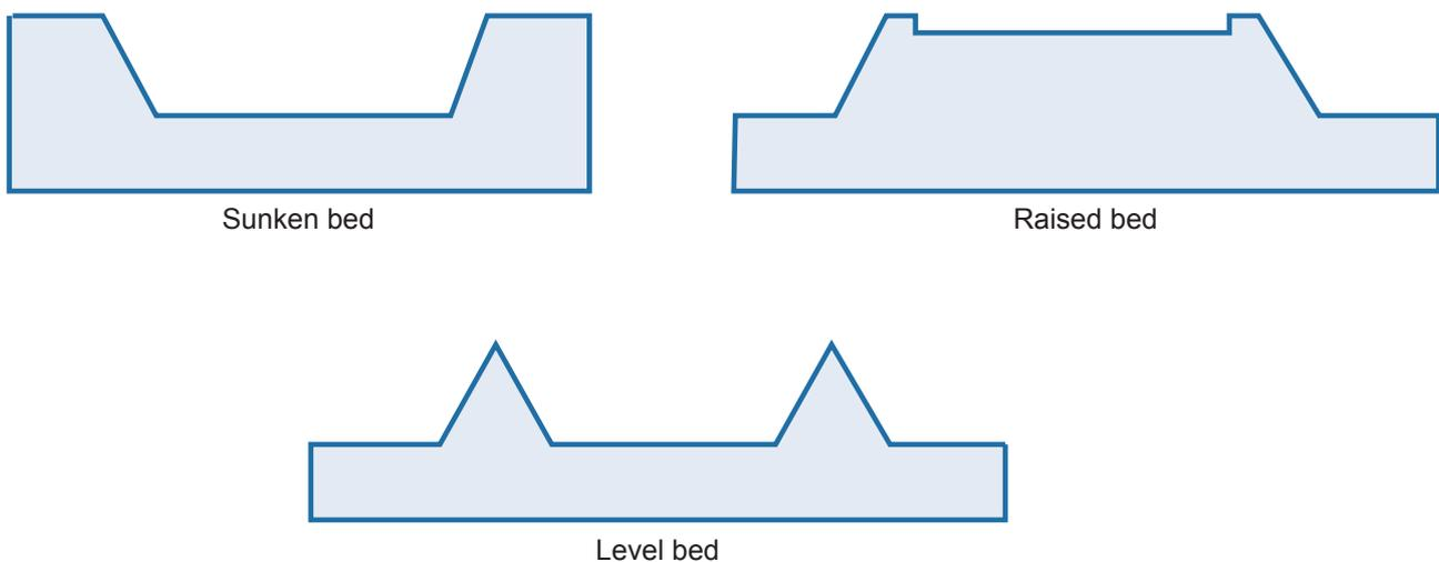
**Figure 3.2 Sunken, raised and level beds**
