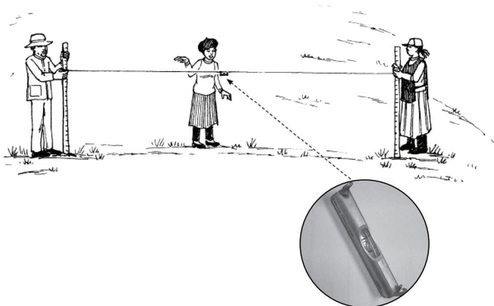
**Figure 3.5** Using a line level to mark contours.
