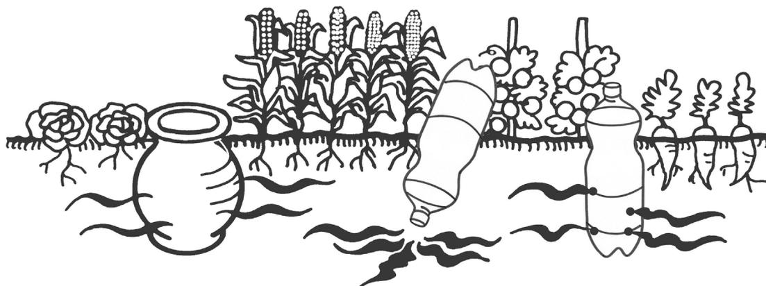
Figure 3.9 Drip bottles for irrigation
